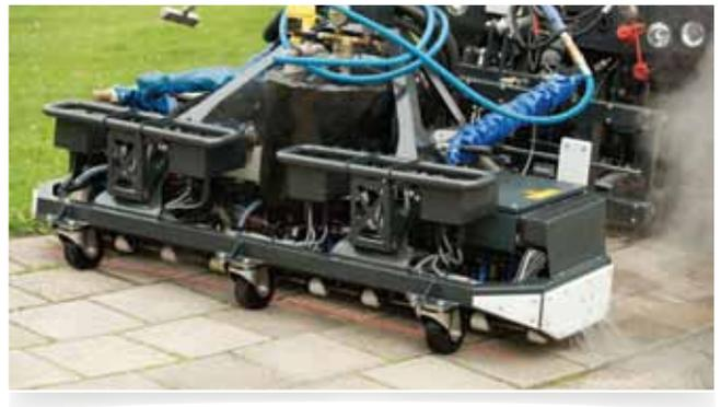
Targeted weed control through detection with sensors.
